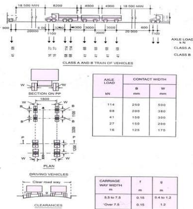
Fig. IRC Class A and B Loadings
