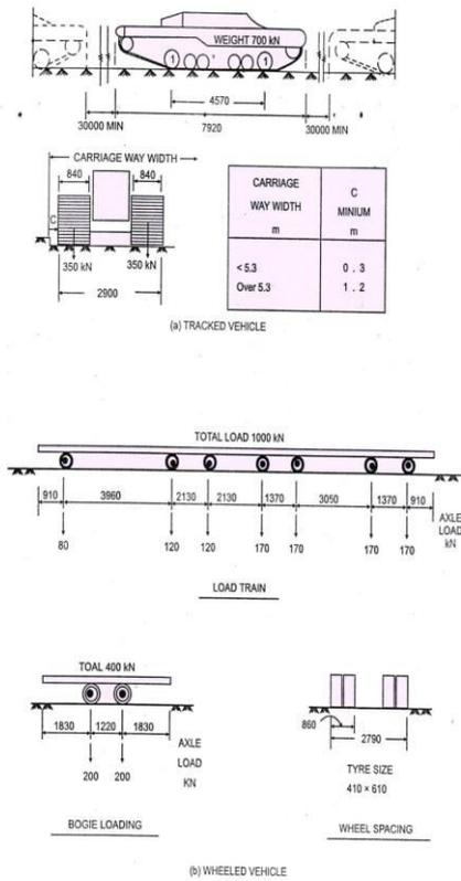
Fig. IRC Class 70R Loading.
